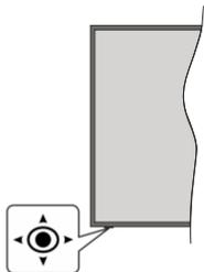
This TV has a joystick as shown in the above drawing. It allows you to control the Volume / Programme / Source and Standby-On functions of the TV.
