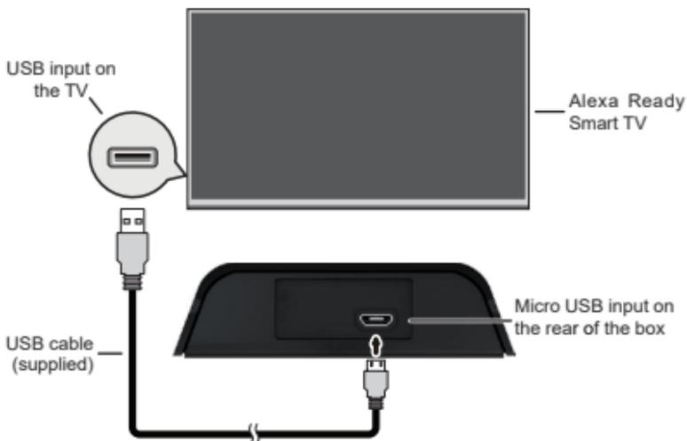
Connect your box to your Alexa Ready Smart TV using the supplied USB cable as shown above. Make sure that your TV is connected to a network with internet access.
