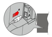
Plug one end (the two-hole plug) of the supplied detachable power cord into the power cord inlet on the rear side of the TV as shown above. Then plug the other end of the power cord into the mains socket outlet. The TV will switch on automatically.
