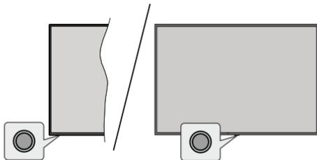
The control button allows you to control the Quick Standby-On function of the TV.
