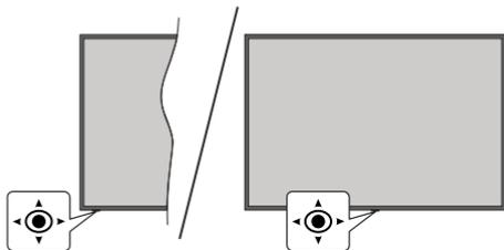
The joystick allows you to control the Volume / Programme / Source and Quick Standby-On functions of the TV.
