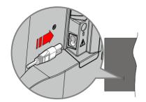
Plug one end (the two-hole plug) of the supplied detachable power cord into the power cord inlet on the rear side of the TV as shown above. Then plug the other end of the power cord into the mains socket outlet. The TV will switch to standby mode.
