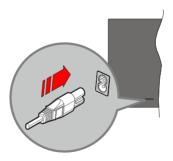
Plug one end (the two-hole plug) of the supplied detachable power cord into the power cord inlet on the rear side of the TV as shown above. Then plug the other end of the power cord into the mains socket outlet. The TV will switch to standby mode.
