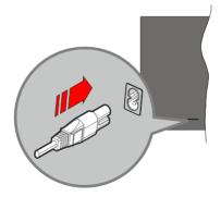
Plug one end (the two-hole plug) of the supplied detachable power cord into the power cord inlet on the rear side of the TV as shown above. Then plug the other end of the power cord into the mains socket outlet. The TV will switch to standby mode.
