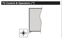
This TV has a joystick as shown in the above drawing. It allows you to control the Volume / Programme / Source and Standby-On functions of the TV.
